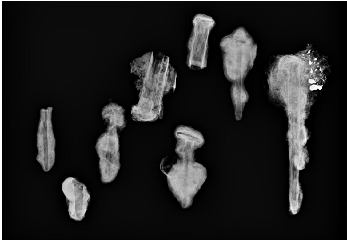
FIGURE 29. X-ray of several concreted fasteners from the Soldier Key Wreck showing the diversity of fastener types used. (Image by author, 2013.)
