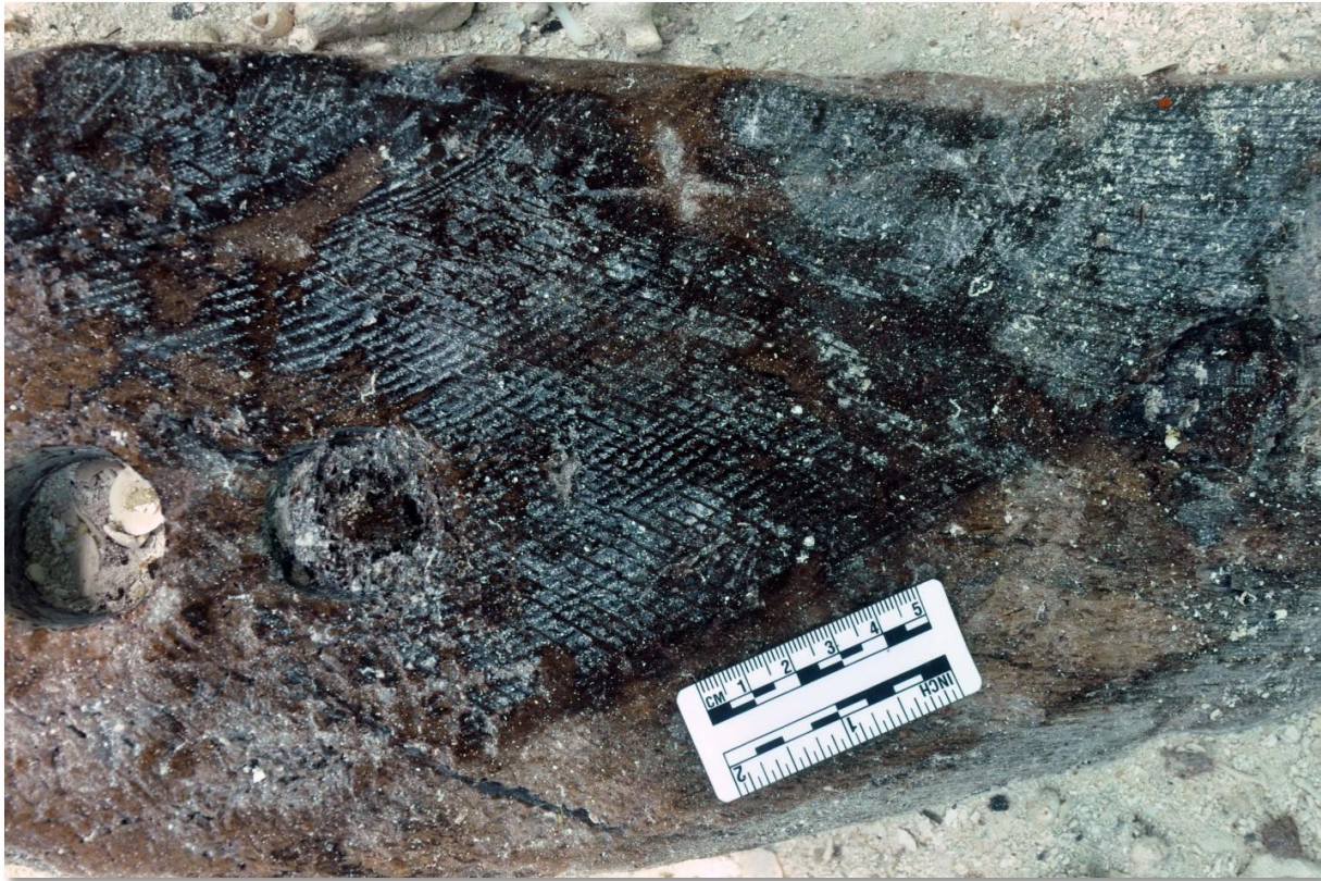
FIGURE 15. Saw marks on the proximal end of second futtock number two. (Courtesy of the National Park Service, 2012.)
